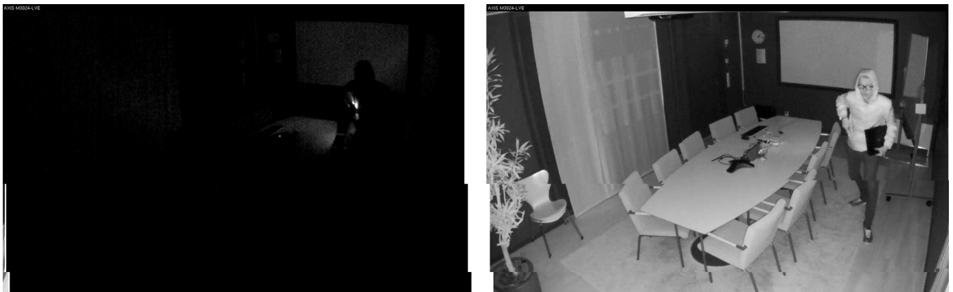
The above images from AXIS M3024-LVE—depicting the same scenario of a man with a small flashlight in a dark room—show the difference that IR illumination makes for surveillance in the dark. The image at left is without the use of IR illuminators. The image at right uses IR light from the camera's built-in IR LEDs. IR light is invisible to the human eye but visible to the camera.
