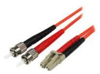
The 50FIBLCST1 1m LSZH LC to ST Fiber Cable features 50/125 micron fiber for high-speed, high bandwidth data transmissions over Gigabit Ethernet and Fiber Channel networks, with support for duplex multimode applications.
