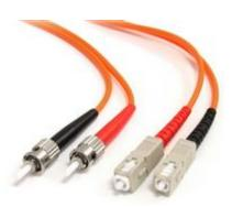
The FIBSTSC2 2-meter (6.6ft) Multimode 62.5/125 Duplex Fiber Patch Cable is terminated with one ST (male) connector and one SC (male) connector, to provide the necessary connection between fiber networking devices for high-speed, long distance networks.
