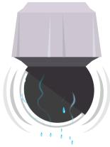
The Sharpdome technology includes Axis' unique Speed Dry function that helps to provide sharp images in rainy weather. It also simplify dome cleaning, allowing for more efficient methods such as high pressure cleaning. With the Speed Dry function activated, the dome vibrates at high speed. It breaks the surface tension of the water and removes the drips.
