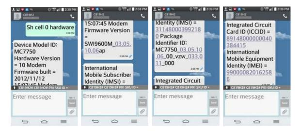
Below is an example of a display command (show cell radio) and a portion of the replies.
