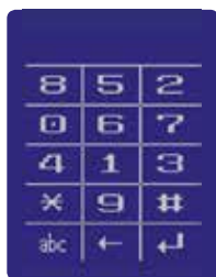
Rotating Keypad (To Prevent Surface Analysis)
