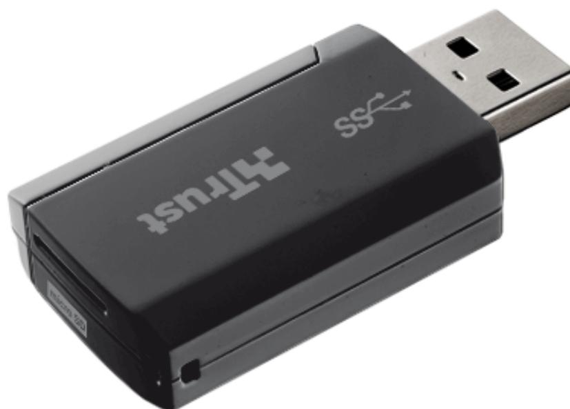
Ultra small and super-fast USB 3.0 SD card reader with extra micro-SD slot
