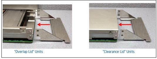
Install (4) M3 x 6mm Flat Head Screws; torque = 6inch-lbs, shown in Figure 3-28.
