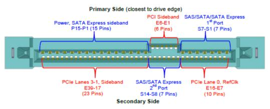
**Note:** 2.5-inch connector supports built in latching capability.
