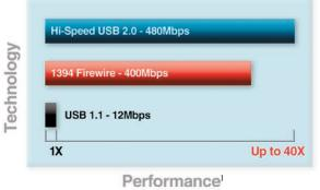
The DUB-H7 performs up to 40 times faster than USB 1.1 by utilizing the 480Mbps<sup>1</sup> throughput speed of Hi-Speed USB 2.0.
