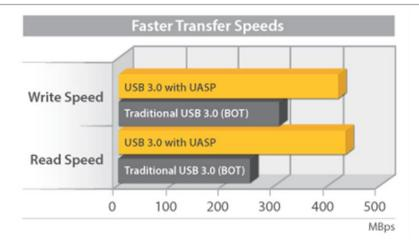
At the same peak in testing, UASP also showed up to an 80% reduction in required processor resources.
