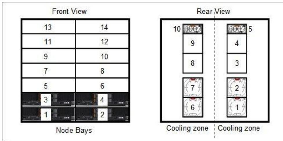
Figure 13. Fan module locations and cooling zones
