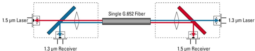
The GLC-BX-D and GLC-BX-U SFPs also support digital optical monitoring (DOM) functions according to the industry-standard SFF-8724 multisource agreement (MSA). This feature gives the end user the ability to monitor real-time parameters of the SFP, such as optical output power, optical input power, temperature, laser bias current, and transceiver supply voltage.
