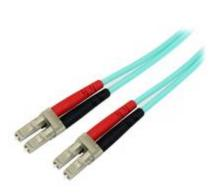
The A50FBLCLC1 1m 850nm Laser-Optimized Multimode Fiber (LOMMF) Aqua Cord features 50/125 micron fiber for high-speed, high bandwidth data transmissions over 10 Gigabit Ethernet and Fiber Channel networks - the perfect solution for fiber cable runs between multiple backbone switches, hubs and routers as well as higher end networking equipment.
