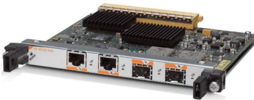
In addition to the two Small Form-Factor Pluggable (SFP)-based Gigabit Ethernet ports, two additional built-in RJ-45 ports are provided on the 2-port Gigabit Ethernet SPA, Version 2. A combination of these Gigabit Ethernet ports is permitted, limited to a total of 2 Gigabit Ethernet ports (both copper, both optical, or one copper and one optical).
