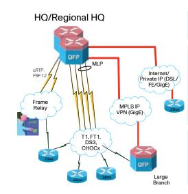
Service provider edge: Layer 3 VPN (L3VPN) provider edge: Example: Distributed provider edge, or provider edge in global VPN networks for bandwidth demands such as asymmetric DSL (ADSL), T1/E1, STM-1, STM-4, Fast Ethernet, Gigabit Ethernet, etc.
