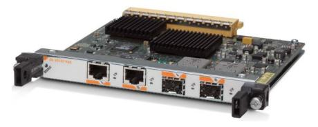
In addition to the two Small Form-Factor Pluggable (SFP)-based Gigabit Ethernet ports, two additional built-in RJ-45 ports are provided on the 2-port Gigabit Ethernet SPA, Version 2. A combination of these Gigabit Ethernet ports is permitted, limited to a total of 2 Gigabit Ethernet ports (both copper, both optical, or one copper and one optical).
