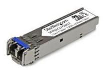
The SFPGLCLHSMST Cisco Compatible Gigabit Fiber SFP Transceiver Module SM LC – 10 km (6.2 miles) is built to comply with MSA (Multi-Sourcing Agreement) standards to offer a cost-effective way to add, replace or upgrade a Single-Mode LC port on your Gigabit fiber networking equipment or fiber media converter.
