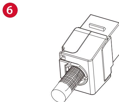
Assemble the keystone jack on face plate or patch panel - this doesn't require excess pressure
