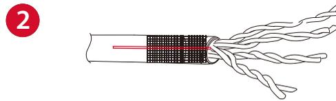
Sandwich drain wire between 2 layers of the supplied foil and then trim any excess
