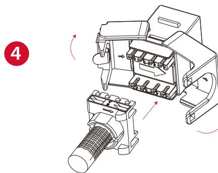
Position the termination cap on the keystone IDCs, in the correct orientation using the arrows
