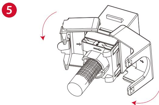
Push the termination cap down and then close the wings
