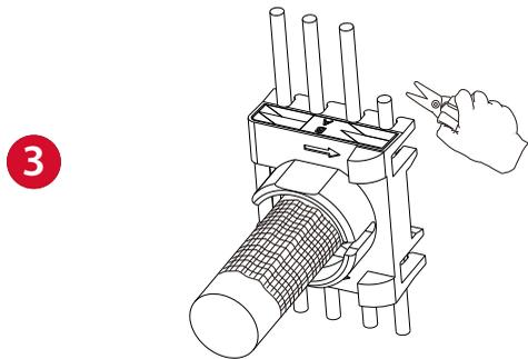
Insert the cable through the termination cap ensuring the cap fits just on the end of where the cable is stripped back to, untwist the four pairs and fan out. Following the colour code on the cap, insert the wires into their designated slots. Double check the wires are in the correct positions and then trim off the excess
