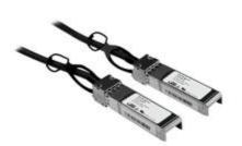
The SFPCMM3M Cisco Compatible 3m SFP+ cable is a fully hot pluggable, direct attach cable, supporting 10 Gigabit Ethernet and Fiber Channel applications connected through (Small Form Factor Pluggable) SFP+ ports.
