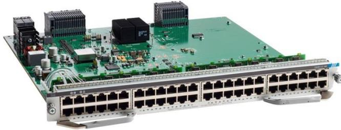
The UPOE line card supports PoE, PoE+, and Cisco UPOE to deliver 15W, 30W, or 60W to the access point. 60W of inline power can power more devices—including IP phones, IPTVs, surveillance cameras, virtual desktop clients, and many others—without having to install extra wall or ceiling circuits while taking advantage of advanced power management capabilities such as Cisco EnergyWise.
