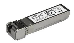
This 10GBase-BX (upstream) SFP+ module delivers what you need most in your network connections: reliable performance. It's built to exacting MSA specifications and fully tested to ensure seamless compatibility. The single-mode SFP+ transceiver module offers a cost-effective way to add, replace or upgrade the ports on your networking equipment, and it's backed by a lifetime warranty.
