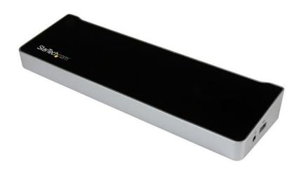
This USB-C<sup>™</sup> docking station for MacBook and Windows® laptops takes productivity to a whole new level, with support for triple 4K monitors - a first in the market. The triple 4K docking station supports Ultra HD 4K resolution on two DisplayPort monitors (at 60Hz), and on one HDMI monitor (at 30Hz).
