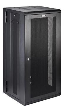
This 26U server or network rack cabinet lets you mount your EIA-310 compliant equipment to the wall, in a secure enclosure that has a hinged rear door for easy access to your equipment. The enclosure features adjustable mounting depth from 3 to 20 in. to provide a robust storage solution for your rack-mount equipment.
