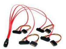
The SAS808782P50 Mini SAS to SAS cable (50cm) features one 36-pin SFF-8087 plug, which fans out to four individual 29-pin SFF-8482 receptacles, providing a reliable solution for connecting multiple SAS HDD drives (with both data and power) to a single mini SAS controller connection.
