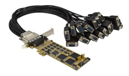
This PCI Express serial card adds 16 high-speed RS232 ports to your standard or low-profile desktop or server PC. This lets you maximize the number of available DB9 RS232 ports that are available for connecting your serial-based devices and equipment, while using only a single PCI Express (PCIe) slot. It's the perfect solution for adding the serial ports you need, even if your desktop PC or server only has a limited number of PCIe expansion slots.
