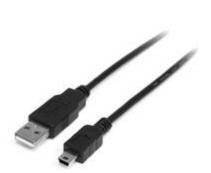
The USB2HABM50CM 0.5-meter (50cm) USB 'A' to Mini 'B' Cable provides one (4-pin) USB Type 'A' male connector and one Mini 'B' (5-pin) male connector, with support for high-speed USB 2.0 transfer rates up to 480Mbps.
