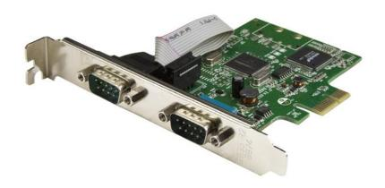
This PCI Express serial card adds two high-performance RS232 serial ports to your desktop computer or server, for connecting your serial-based devices and equipment.
