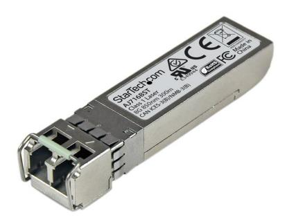
This HP® compatible 8 Gigabit Fibre Channel Short Wave SFP+ is engineered by StarTech.com to deliver what you want most in your network connections: reliable performance. Built to exacting specifications and fully tested to ensure maximum performance, you can install this high-quality fiber transceiver module into HP networking devices that support the HP AJ716B FC SFP+ transceiver module, as well as other major brands of networking equipment.
