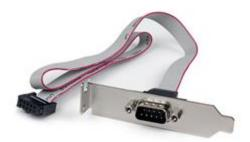
The PLATE9M16LP (16 inch/ 0.4 m) Low Profile Serial Plate adds a DB9 serial port to the rear panel of a small form factor/low profile computer, connecting to an IDC10 header connector on the motherboard.
