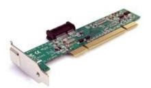
The PCI1PEX1 PCI to PCI Express Adapter card lets you use low profile PCIe expansion cards in a server/desktop motherboard PCI slot. The adapter connects through a 32-bit PCI slot to provide a low profile PCIe x1 slot in its place; a spare, full size bracket is included for installation in larger desktop or server expansion slots that can accommodate a full-sized card.
