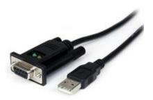
The ICUSB232FTN FTDI USB to Null Modem Serial Adapter Cable (1-Port) converts an available USB 1.1 or 2.0 port into an RS232 Null Modem serial DB9 port, solving DCE/DTE conflicts directly, without requiring additional cross-wired serial cables or adapters.
