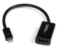
The MDP2HD4KS Mini DisplayPort to HDMI adapter enables you to connect a mDP-equipped Ultrabook™, tablet or laptop computer, such as the ThinkPadT440 series, to an HDMI display. This adapter is compatible with Mini DisplayPort 1.2 & HDMI 4K @ 30 Hz and as a result can support video resolutions up to Ultra HD (4K) as well as the accompanying digital audio up to 7.1 channel surround sound.
