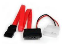
The SLSATAF12 Slimline SATA to SATA with LP4 Power Cable (12-inch) features a SATA data receptacle and a Molex (LP4) power connection on one end, and a Slimline Serial ATA receptacle on the other - allowing you to connect a slim SATA drive to a computer motherboard that does not have a Slimline connection available.
