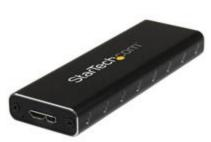
The SM2NGFFMBU33 external USB 3.0 to M.2 (NGFF) enclosure turns your SATA M.2 solid state drive into a portable, high speed USB 3.0 drive.
