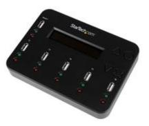
The USBDUP15 OnetoFive USB flash drive duplicator and eraser lets you quickly clone up to five backups of a single USB flash drive, or securely erase up to six flash drives, without connecting the to a host computer.
